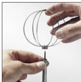
5) Keep ring nut fixed, insert and screw down the thread protection.
