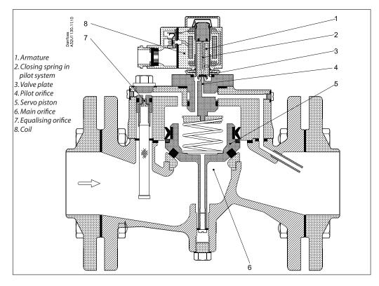
Coil voltage disconnected (closed):
