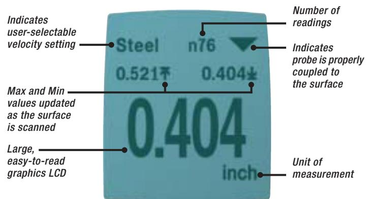
**UTG ME model** features Thru-Paint capability to quickly and accurately measure the metal thickness of a painted structure without having to remove the coating. The most accurate method to measure remaining wall thickness of a painted structure because it automatically disregards the coating, lowering inspection time and expense. Also ideal for measuring on sandblasted materials or other applications requiring a more durable wear face.
