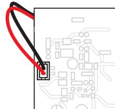
The probe and its lead should **NEVER** be installed in ducting along with power, control or power supply wiring. Always disconnect the power supply when making the connections.
